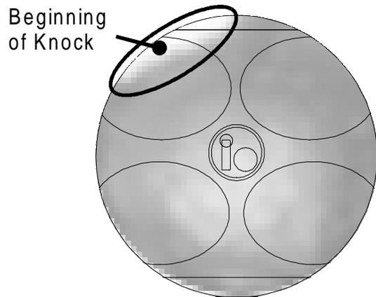
Figure 12: Beginning of knocking combustion with variation of the inlet flow (tumble shield 5°)
