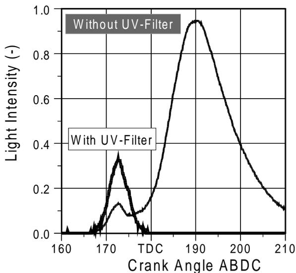
Figure 8: Light signals with different spectral response
