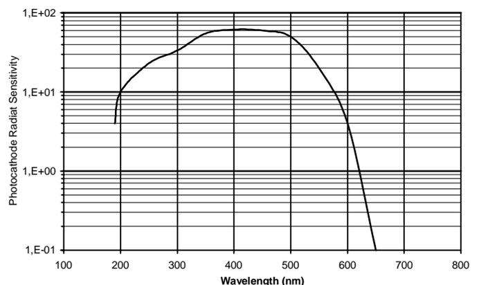
Figure 4: Spectral response of PMTs
