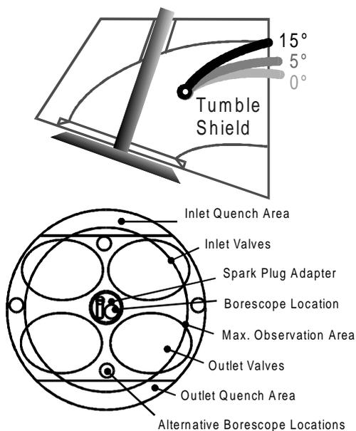
Figure 6: Cylinder head arrangement
