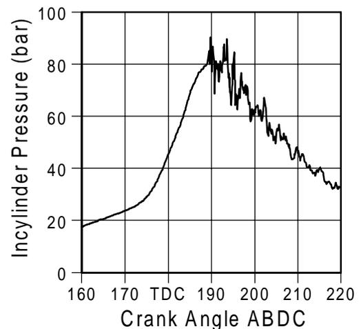
Figure 9: Signal course of a knocking combustion
