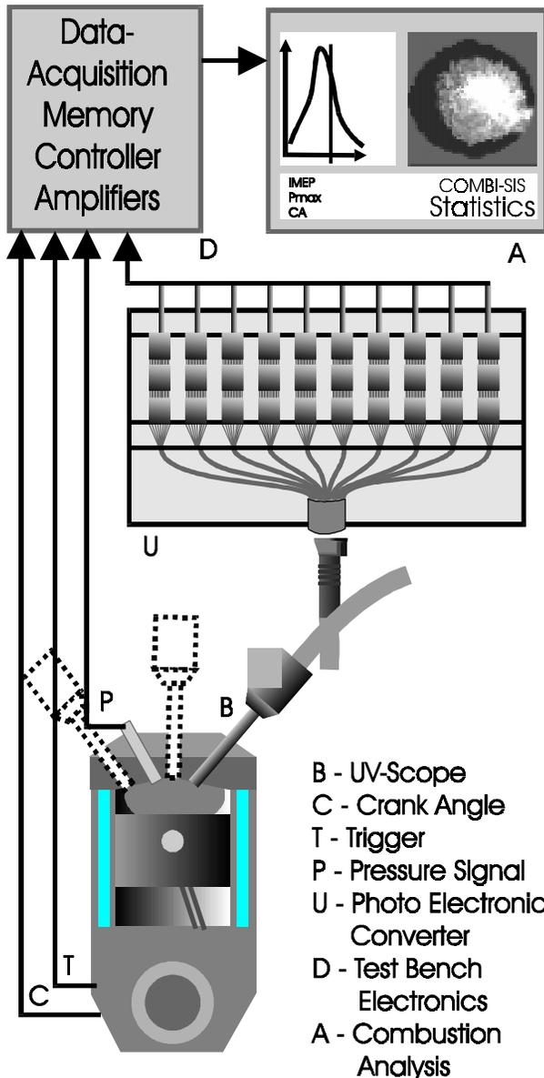
Figure 1: Flow chart of the experimental setup
