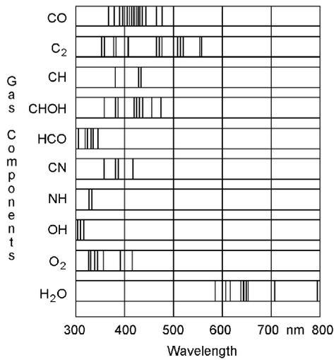
Figure 5: Spectral bands of HC-Combustion in SI-Engines
