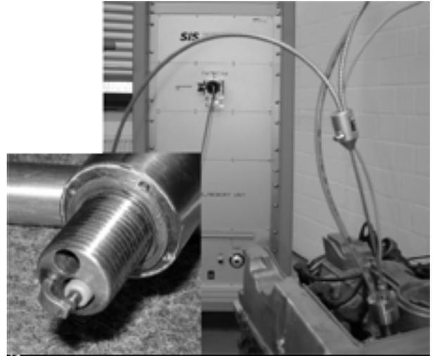
Figure 7: Spark plug adapter and test bench view
