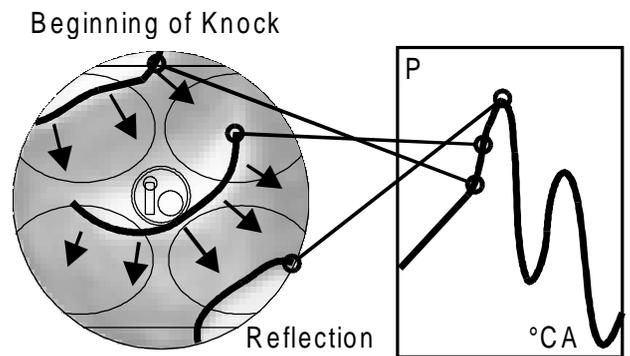
Figure 13: Spreading out of pressure waves after initial knocking
