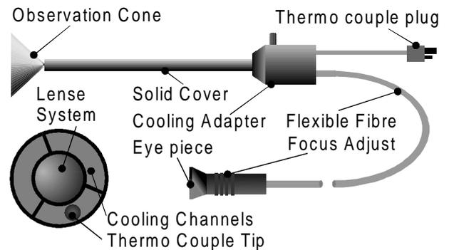
Figure 2: UV-Scope - Components and Front View
