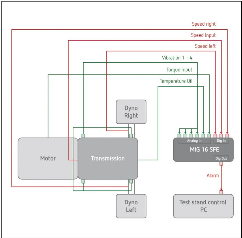
**Figure 4:** Signals to connect a SFE measurement system to a power train test bed.
