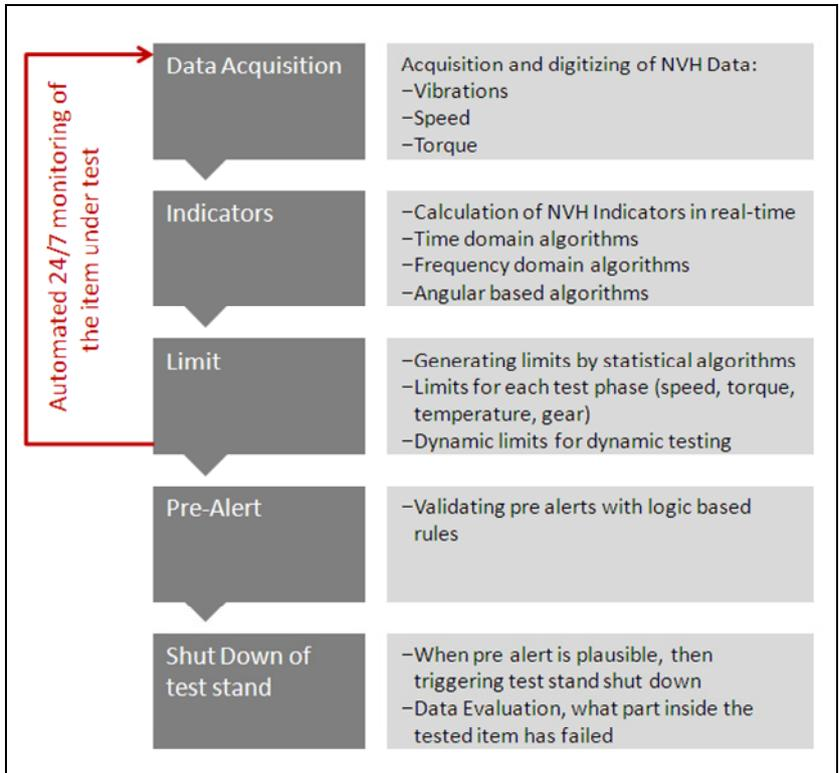
**Figure 5:** Process of SFE from data acquisition through to shutdown of the test bed.
