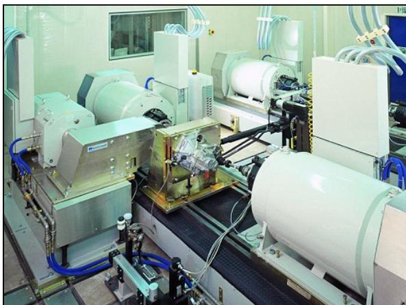
**Figure 1:** Power train test bed for testing of transmissions and axle drives.
