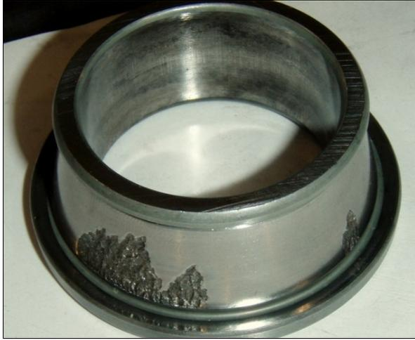
**Figure 8:** Damage to the inner ring of the pinion head bearing of an axle transmission. Pitting size about 25 mm<sup>2</sup> and 5mm<sup>2</sup>.
