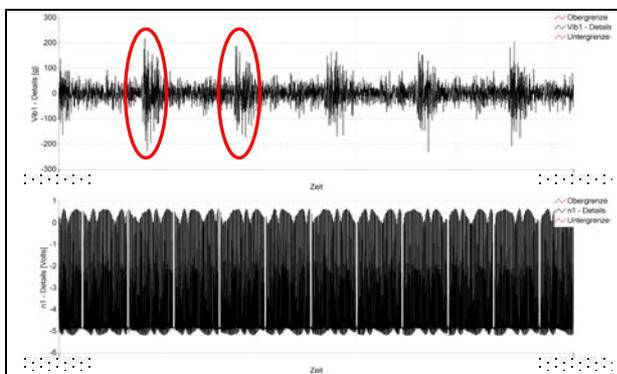
**Figure 10:** Top graph vibration acceleration as 24 bit/50 kHz Signal. Crankshaft angel signal from the 60-2 engine speed sensor.
