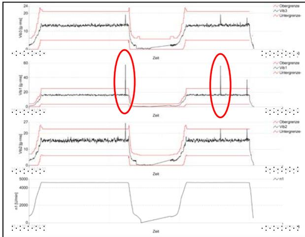
**Figure 12:** Top-Down: Lapse of MIG16 NVH-Indicator on crankshaft housing, cylinder head 1,2 , cylinder head 3,4, crank shaft speed
