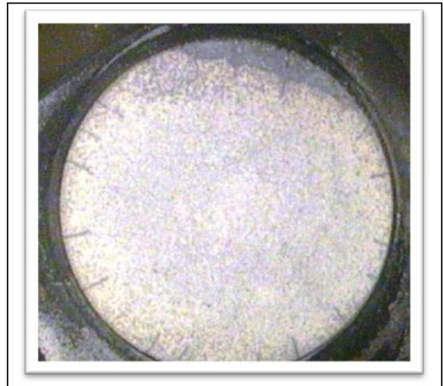
**Figure 14:** Endoscopy of the combustion chamber is revealing the MIG16 diagnosed damage: radial cracks on the exhaust valve of cylinder 2.
