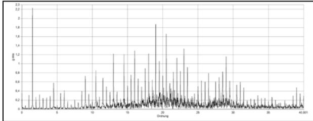
**Figure 7:** high resolution 3D- and 2D-orderspectrum of a combustion engine durability test.
