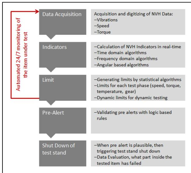
**Figure 2:** Process of the data acquisition and NVH-indicator calculation of MIG16
