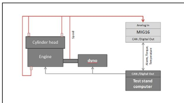
**Figure 3:** Signals for a MIG16 system at an engine durability test stand
