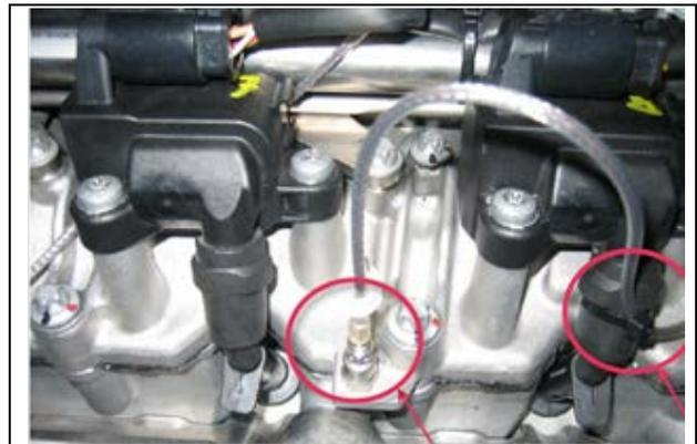
**Figure 4:** Location of the vibration sensors at the cylinder head
