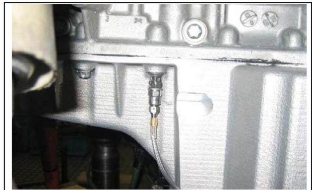
**Figure 5:** Location of the vibration sensors at the crankshaft housing
