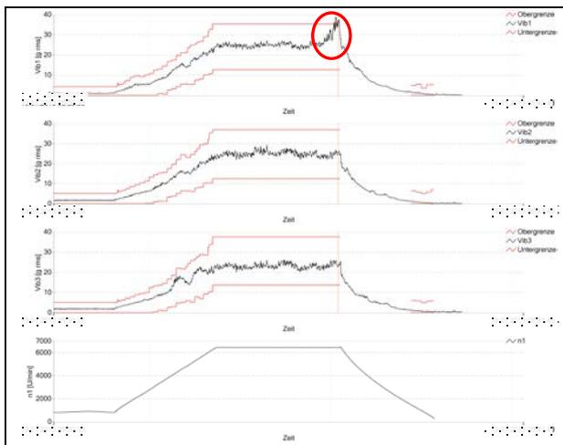
**Figure 9:** graph 1-3 are showing the MIG16 RMS NVH-indicator on crankshaft housing, cylinder head close by cylinder 1 and cylinder head close by cylinder 3. Graph 4 shows the speed of the engine during the test.
