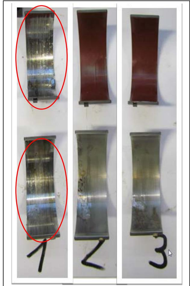
**Figure 11:** bearing half shelves for the 3-cylinder engine after a MIG16 shut off. Bearing number 1 shows clear abrasive marks.
