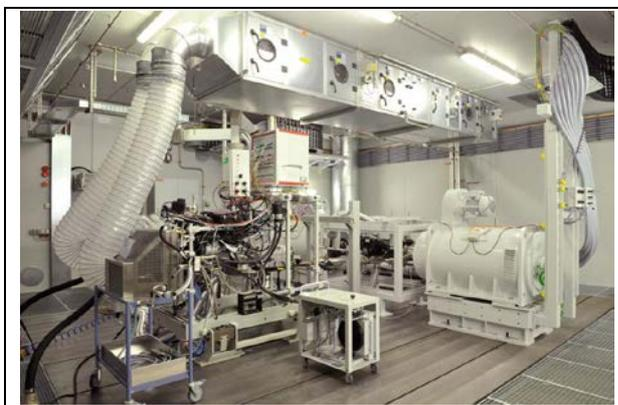
Figure 1: test stand for durability testing of combustion engines
