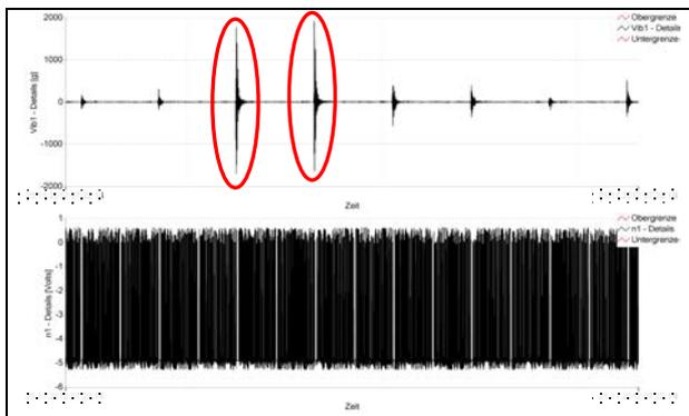
**Figure 13:** Details of the MIG16 measurement data close to the vibration event on cylinder number 1 and 2.
