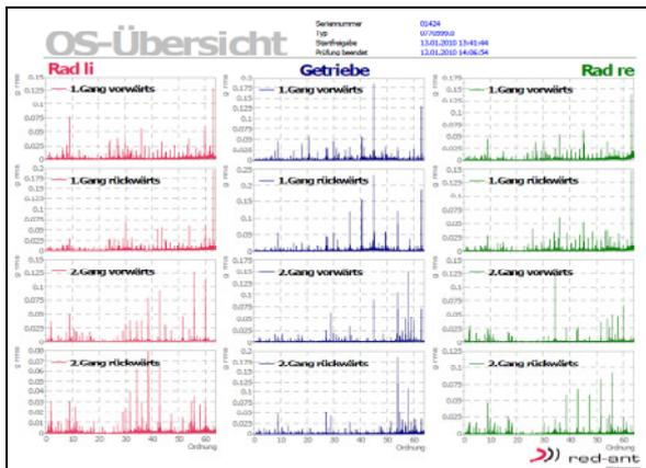
Figure 5: NVH-order spectrum indicator for a manual gearbox with a flange attached axle.
