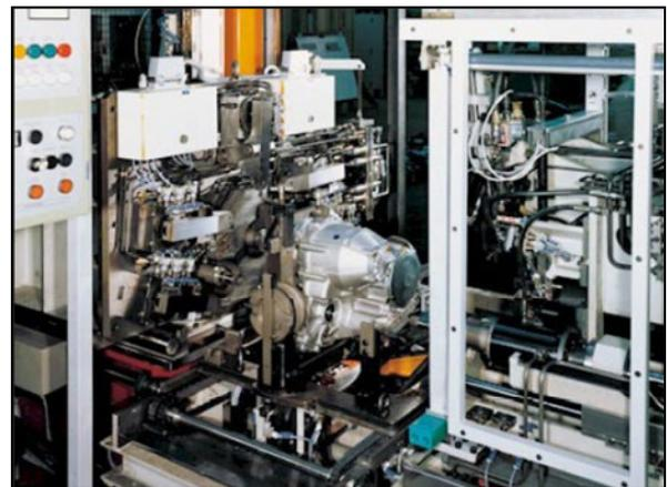
**Figure 1:** Test bed for acoustic quality control for automatic transmissions.
