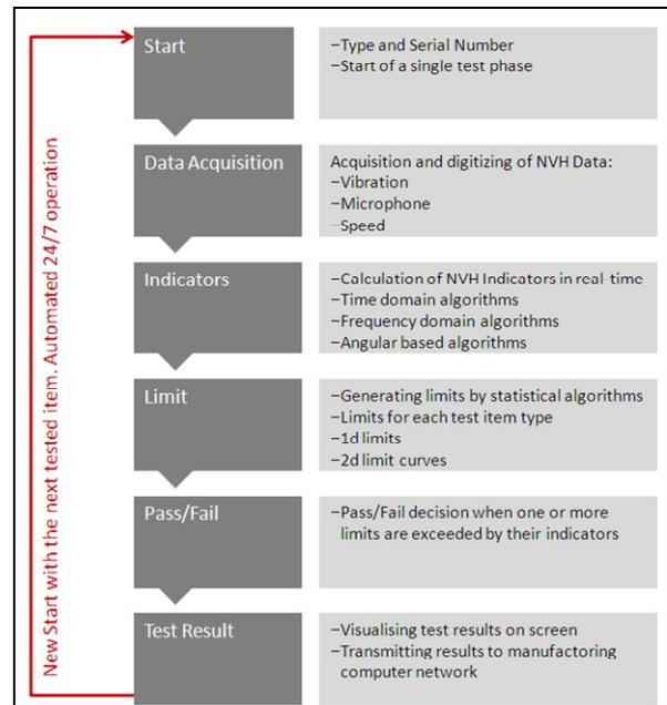
**Figure 4:** Course of events diagram of an AQS-measurement system on an end-of-line test bed for functional and noise testing of engines, transmissions and axle drives
