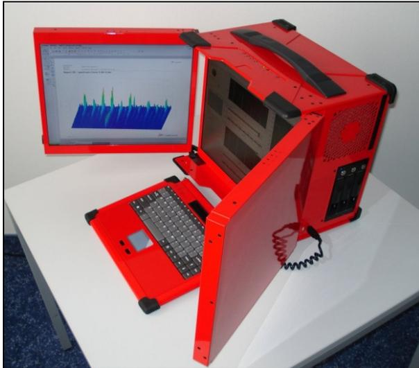
**Figure 2:** MIG16 measurement system for acoustic quality control (picture shows a portable version for measuring a vehicle, also available as a 19-inch junction box).
