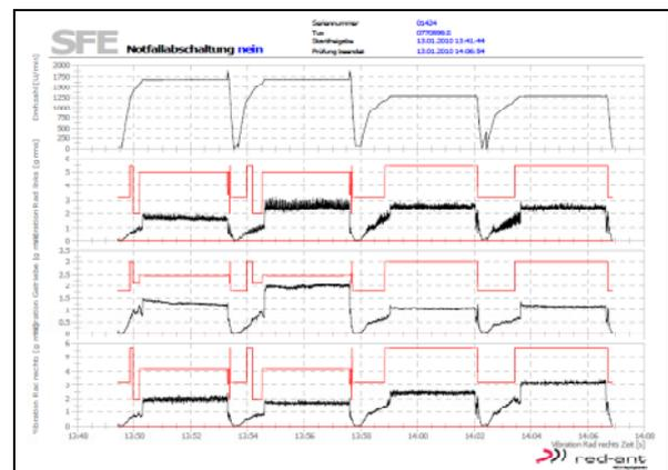
Figure 7: Emergency shutdown after permanent body sound monitoring during the AQS examination of a manual gearbox with a flanged axle. Upper graph: Rotational speed profile during the entire measurement, 1st gear driving, 1st gear braking, 2nd gear driving and 2nd gear braking. Lower three graphs: black line: NVH indicators of different measuring points (top to bottom: left wheel head, manual transmission, right wheel head), red lines: Limit values.
