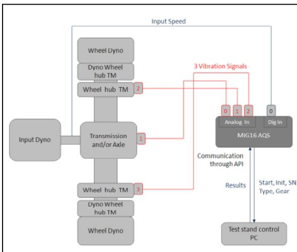
**Figure 3:** Wiring diagram of an AQS-measurement system on an end-of-line test bed for functional and noise testing of transmissions and axle drives.
