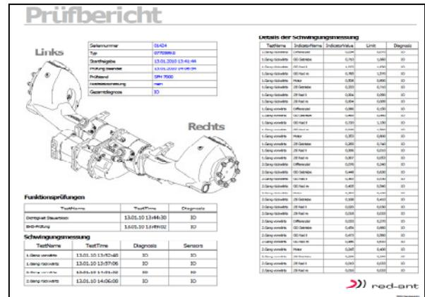
Figure 6: Audit report of the product with serial number, type, date, functional test results, results of vibration measurement in short form (left side) as well as all detailed NVH indicators (table on the right side).
