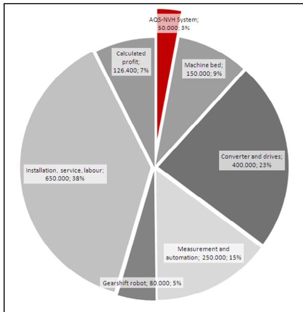
**Figure 8:** Cost of a fully automated manual transmission end-of-line functional test bed for a German manufacturer
